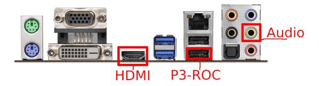
Connect the 24-pin power, SATA cable, HDMI, P3-ROC USB, and analog audio as shown. Install the memory DIMM in the slot shown above. (Slot 1) Connect the other side of the SATA cable to the SSD, and plug power into the SSD.
